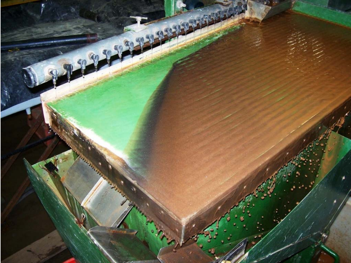
Figure 3: Hole 7 Pass one on Table - cassiterite separating on outer edge followed by magnetite
